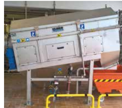
Washing of contaminated grit with the versatile HUBER Wash Drum RoSF9.
