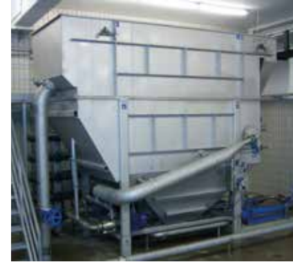
HUBER Dissolved Air Flotation Plant HDF for solids separation in a beverage industry.
