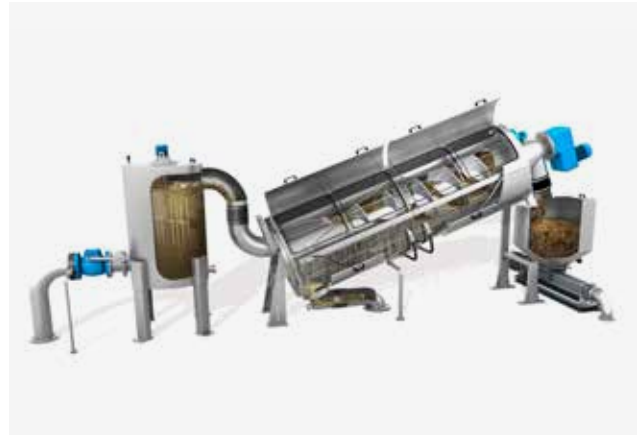
Sectional view of a S-DRUM size 4L.
