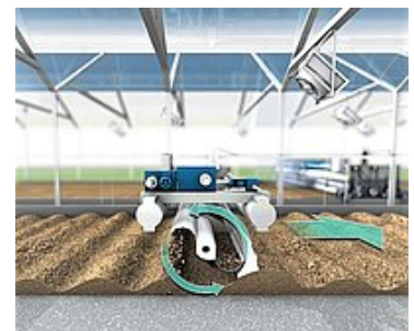
A double shovel is ploughing through the sludge bed and turning the sludge as the machine is moving through the greenhouse
